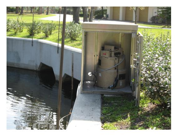
Figure 2-2. Inflow Monitoring Equipment at Site 1.
