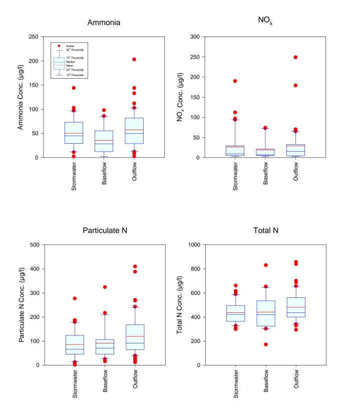
Figure 3-15. Statistical Comparison of Nitrogen Species Measured in Stormwater, Baseflow, and Outflow at the Navy Canal Pond Site.
