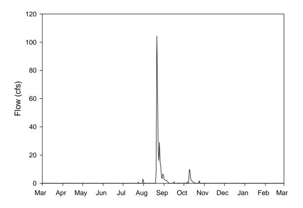
Figure 3-6. Discharge Hydrographs for the Diversion/Spillway Structure (50-ft Rectangular Weir).
