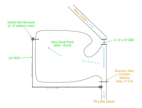
Figure 1-3. Schematic of System Components of the Navy Canal Stormwater Facility.
