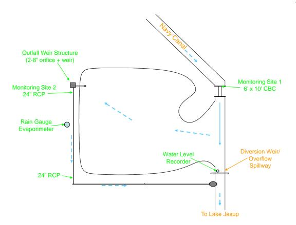
Figure 2-1. Locations for Monitoring Equipment at the Navy Canal Site.
