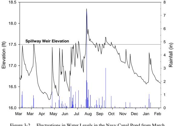
Figure 3-2. Fluctuations in Water Levels in the Navy Canal Pond from March 2008-February 2009.
