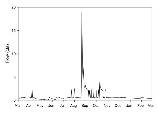
Figure 3-5. Discharge Hydrographs through the Pond Outfall Structure.
