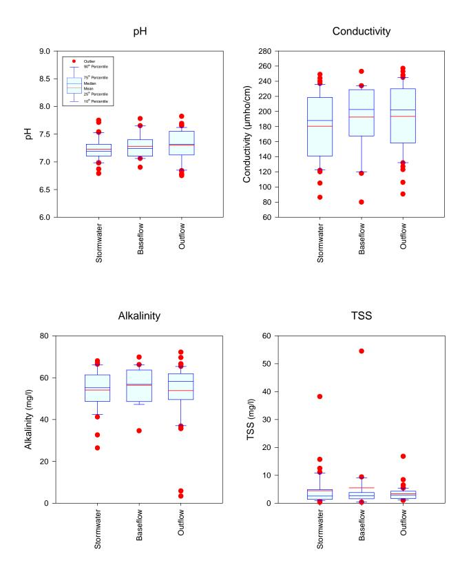
Figure 3-14. Statistical Comparison of General Parameters Measured in Stormwater, Baseflow, and Outflow at the Navy Canal Pond Site.
