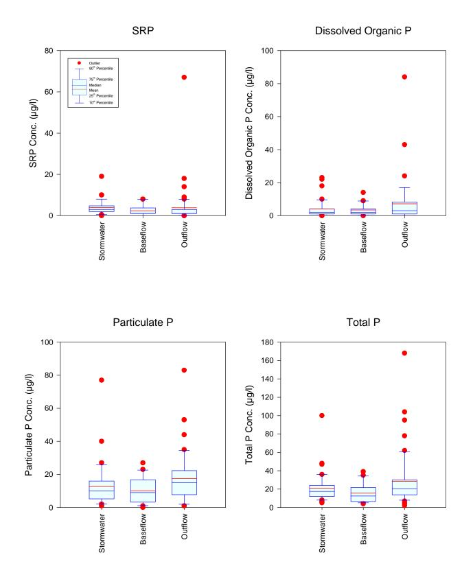
Figure 3-16. Statistical Comparison of Phosphorus Species Measured in Stormwater, Baseflow, and Outflow at the Navy Canal Pond Site.
