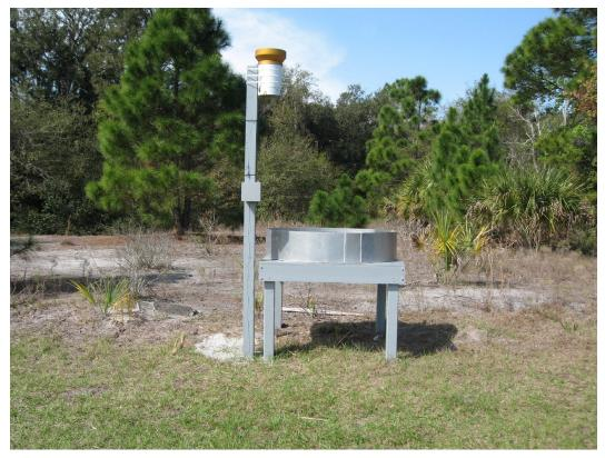
Figure 2-4. Rainfall and Pan Evaporation Equipment.
