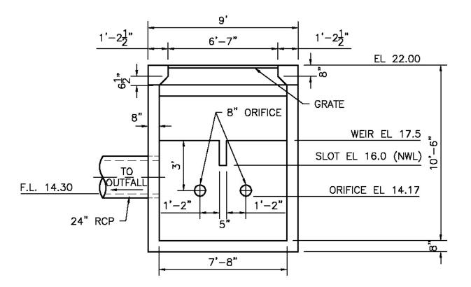
Figure 1-8. Schematic of the Navy Canal Pond Outfall Structure.
