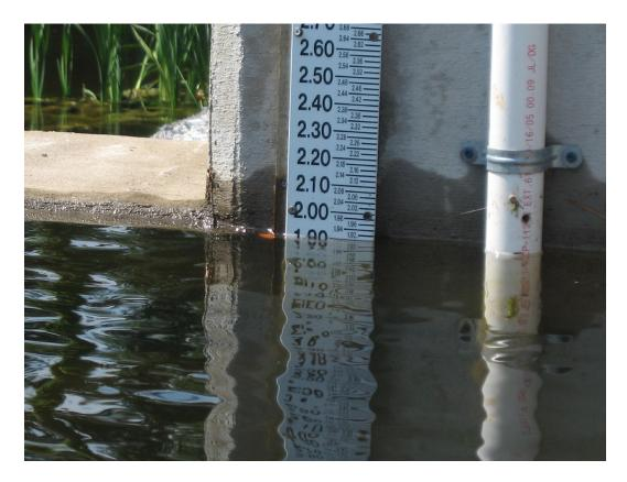
Figure 2-5. Staff Gauge and Water Level Recorder.
